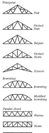
This chart is for steel trusses fabricated from structural steel members. Because these trusses are custom designed and fabricated, a great variety of shapes and configurations are possible.
