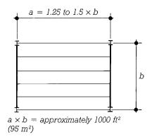
For economical framing of steel bays, the lighter beams should span 1.25 to 1.5 times the span of the heavier girders. Bay area should equal approximately 1000 ft<sup>2</sup> (95 m<sup>2</sup>).
